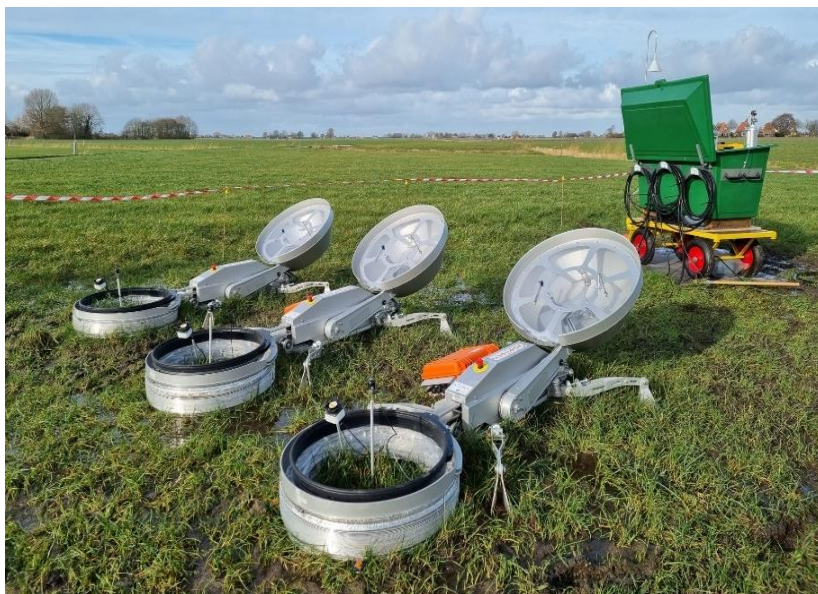
Figure 4. Set up of the three automatic flux-chambers with the manual control boards (orange cases) attached to the side of each chamber. The equipment housing (green cart) containing the sensor and other peripherals was positioned behind the chambers (i.e. not in line with the stable and the chambers). The air inlet for ambient concentration measurements was attached to the equipment housing. On a regular basis fertilizer was applied to the grassland. At the same time the practices within and around the chambers were closely simulated by hand with the same amount and composition of manure and fertilizer.
